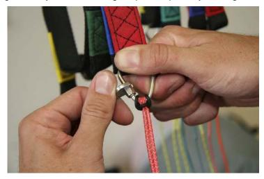
Fig. 7: Closing and tightening the quick link
