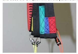
Fig. 12: C1 quick link on the standard riser
