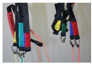
Fig. 9: Paramotor riser with B-quick link (to the right-hand side)
