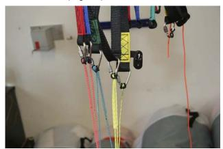
Fig. 14: Paramotor riser with all lines, except the brake line
