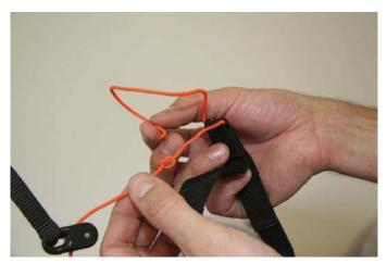
Fig. 15: Brake line with the knot undone
