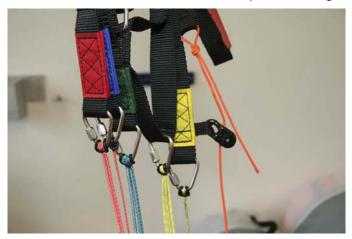
Fig. 22: Paramotor riser with all main lines and brake lines (the right-hand riser is shown here)
