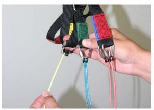
Fig. 11: Paramotor riser with stabiliser lines on C1
