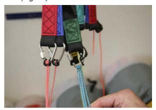
Fig. 10: Paramotor riser with B-lines
